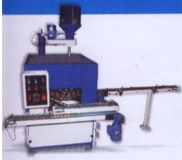
Wedding machine inserts the wads into ready caps. Wads are feed into the machine with the help of Feeder Device through vibrating system.
